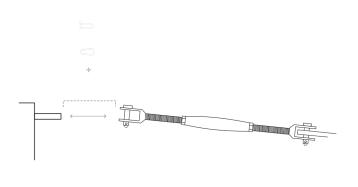
Bridge any gap between Turnbuckle and anchorage points with non-adjustable fixings
